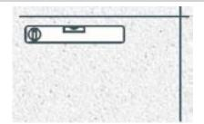
Using a laser or conventional building level, determine the ideal horizontal and vertical lines, mark tem with a pencil
