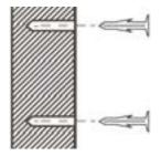
Removing the panel, drill holes at the marked points. In the finished holes, insert the plastic dowels. In the case of mounting at the wall of foam bloacks or plasterboard use the special dowls "Driva" from the set of consumables "Artpole".
